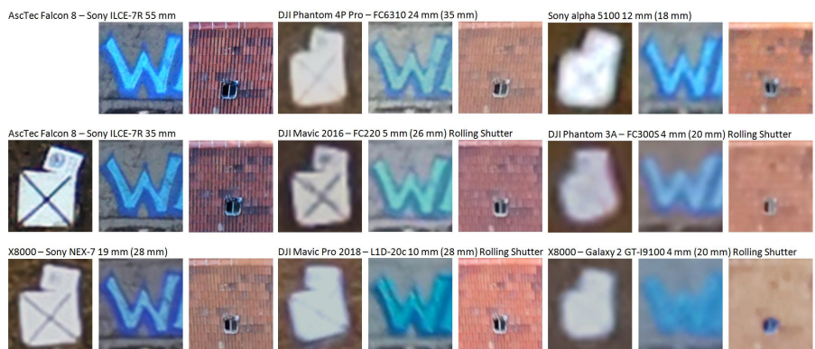
Fig. 5. Samples of imagery for the nine different camera systems: GCP Teflon panel – high contrast, graffiti on roof – low contrast, tiles on roof – fine scale texture.
