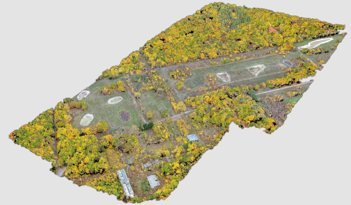
Fig. 4. 3D point cloud of test site delineated based on DJI Mavic Pro 2018 imagery.
